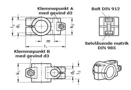
Adjustable clamp lever for d3 = GN 911-M10-55 have to be ordred separately 11 = 122.0Adjustable clamp lever for d4 = GN 911 - M 8 - 32 have to be ordred separately
